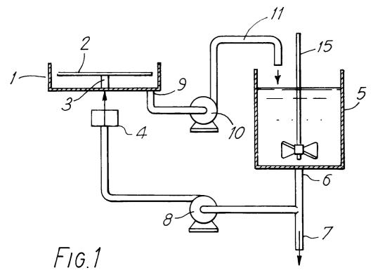
This invention relates to a destruction process and particularly to a process for the decomposition of organic material by ultraviolet light.
