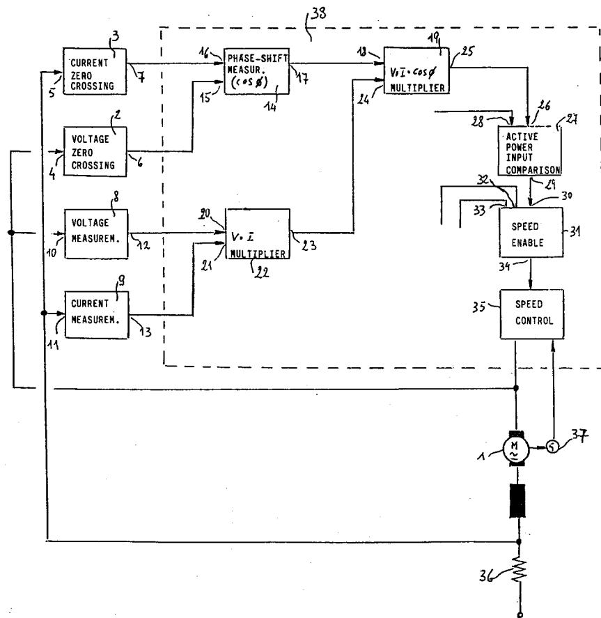
The present invention relates to an electronic arrangement that is provided in washing machines, particularly clothes washing machines and combined clothes washing and drying machines, and is adapted to measure and balance out-of-balance washloads in the drum of such washing machines when performing their laundering processes.
