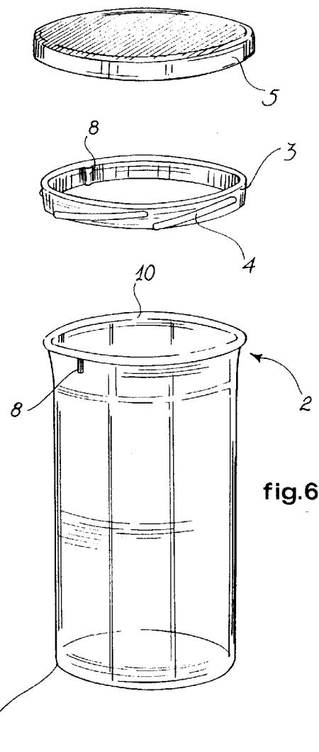
The invention relates to a hermetic closing device for drinking glasses or in general containers for food-stuffs, which device is removable and detachable to permit the application of a cover, of known type, and the hermetic closing of the container and, after the product has been finished, to permit a wider and easier use of the container as a recipient for different applications.
