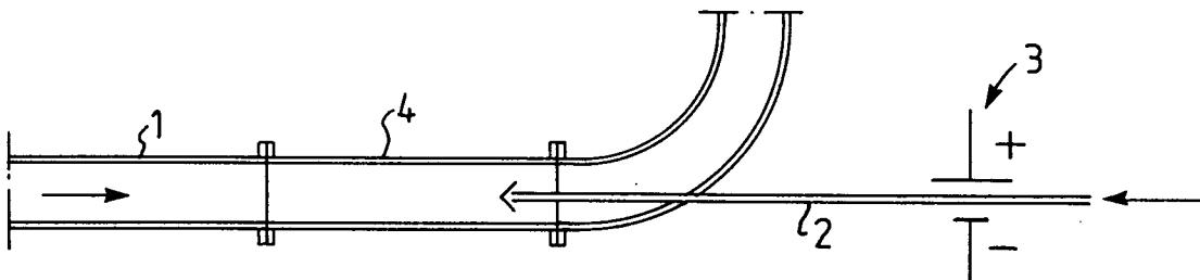
This invention refers to a method and a device for the glue coating of particles, primarily of cellulose material such as fibres and chips, in connection with the manufacture of e.g. fiber board according to the dry method, so-called MDF (Medium Density Fiberboard), dry-formed paper and particle board.
