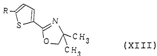
10 wherein R represents an alkyl group having 1 to 4 carbon atoms, with a base such as butyl lithium to produce an ortho-lithiated compound, which is then reacted with a compound represented by the general formula
