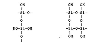
In the silicic acid oligomer (b) prepared from a silicate compound in the above-described manner, OH groups remain on the outer surfaces thereof. As described above, therefore, it is preferable from the viewpoint of miscibility with the silicic acid oligomer (b) to use a radical-polymerizable vinyl compound having a hydrophilic group as the component (a).
