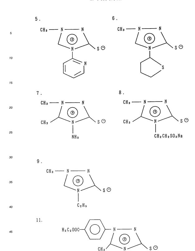
The mesoionic compound is preferably added to the processing solution in a concentration of about  $1 \times 10^{-5}$  to 10 mol/liter, more preferably  $1 \times 10^{-3}$  to 3 mol/liter. Either a single mesoionic compound or a mixture of mesoionic compounds may be used. In the latter case, the total amount of mesoionic compounds falls in the above-defined concentration range.
