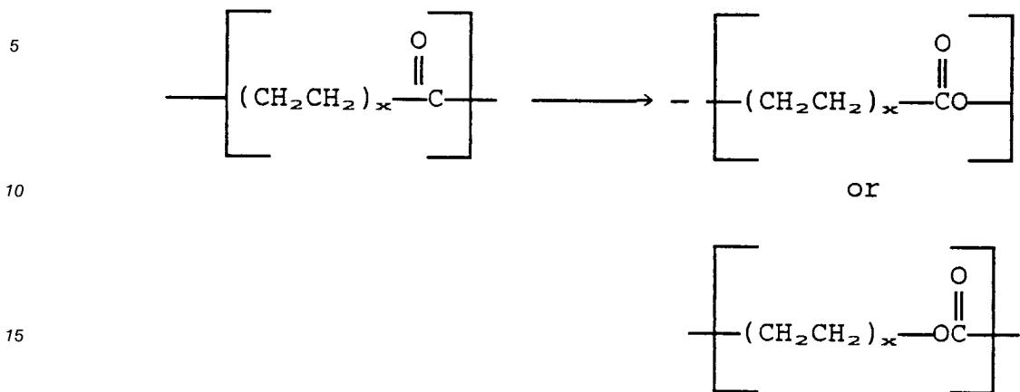
where  $x$  is an integer representing the number of adjoining ethylene units at a particular CO site. As is evident from the above equation, insertion of the oxygen atom can occur on either side of the carbonyl.
