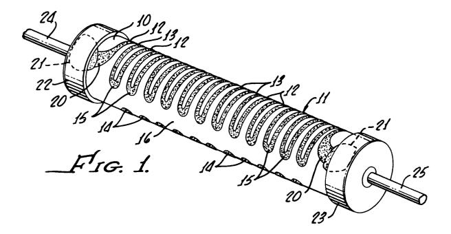
In high-voltage film resistors used for many types of applications, it is very important that there be a low voltage coefficient, it being understood that the voltage coefficient is the variation in resistance that occurs as applied voltage is increased or decreased (but not taking into account the resistance variation caused by self heating of the resistive film).
