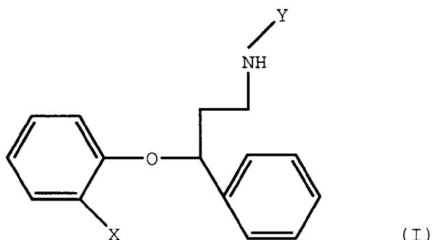
wherein X is C<sub>1</sub>-C<sub>4</sub> alkylthio, and Y is C<sub>1</sub>-C<sub>2</sub> alkyl or a pharmaceutically acceptable acid addition salt thereof.
