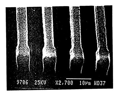
Before Polymer Cure: 4 um imaged polymer lines
