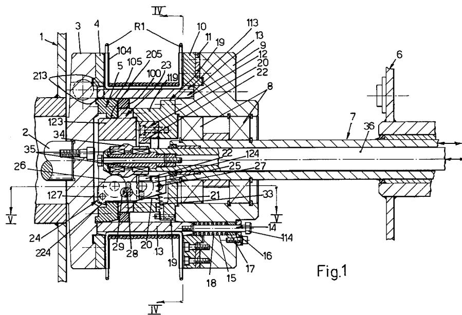
The invention relates to a precision mandrel, particularly suitable for winders which are required to execute windings of the parallel-turn type, in other words windings in which the turns of each layer are placed exactly side by side and in mutual contact, so that the winding is made to be compact and of regular form.
