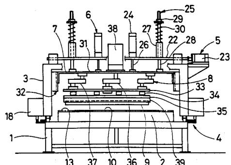
The present invention relates to a method and an apparatus for polishing the surface of a plate such as a metal plate and a non-metal plate, particularly suited for polishing of large-sized plates.
