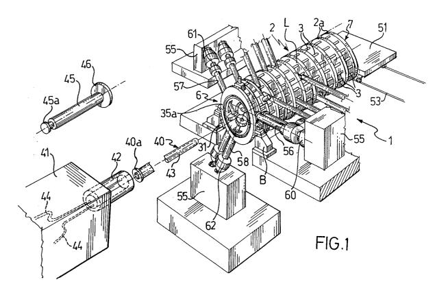
This invention relates to a rolling stand having at least three driven rollers, an outer support structure for said rollers, driving means and associated mechanical transmission means for driving the rollers. said stand being placed along a longitudinal rolling axis.
