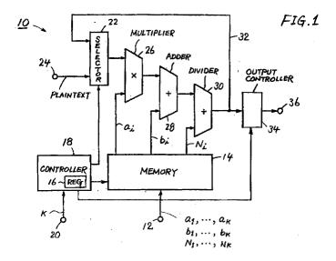
The present invention relates to an arrangement for transforming plaintext into the corresponding ciphertext in a digital data communications system. The arrangement disclosed is also applicable to the reverse process of transforming ciphertext into the original plaintext.
