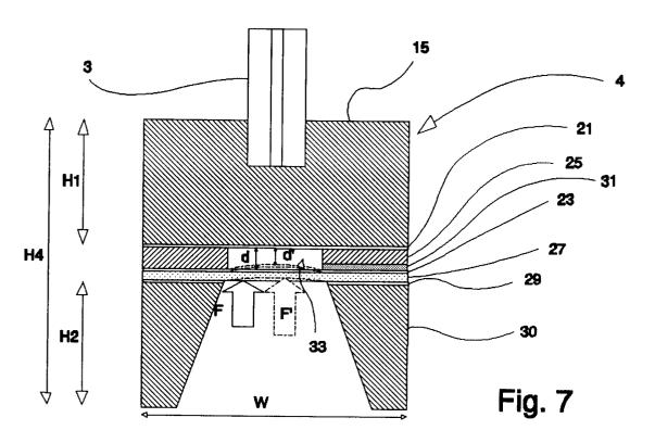
The present invention is related to an optical force transducer according to the preamble of claim 1.
