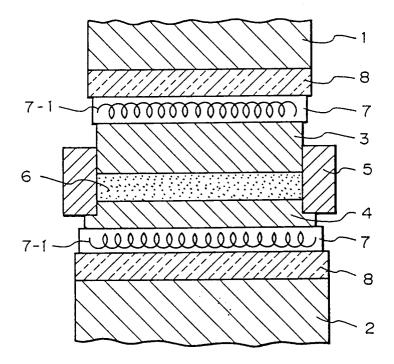
This invention relates to a carbon/metal composite. More particularly, it relates to a carbon/metal composite having a high strength, good wear resistance, and good electrical properties and which is suitable for use as a sliding current collector such as a pantograph slider for electric trains.
