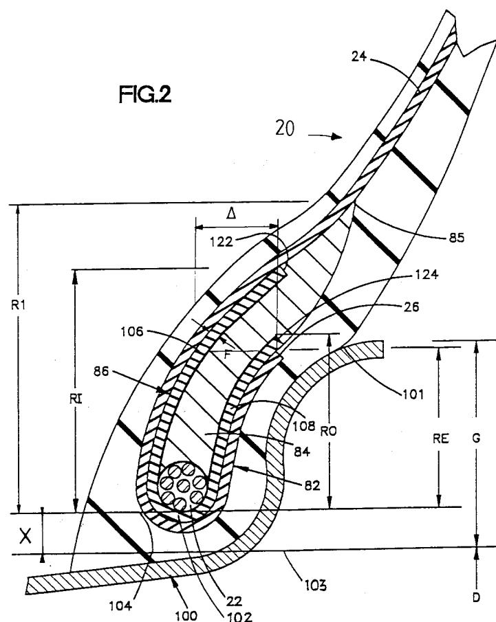
The present invention relates generally to a pneumatic vehicle tire. In particular, the present invention relates to an improved flipper structure in the bead area of the tire.
