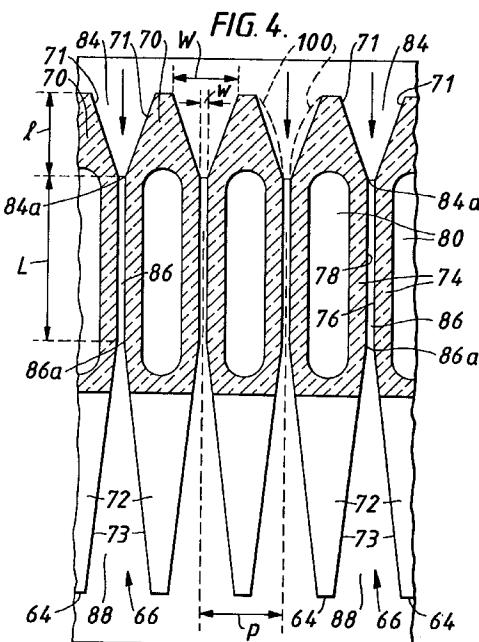
The present invention relates to a fuel fired burner, and particularly a gas-fired burner, which preferably is of the fully premixed type i.e. one in which the fuel gas is mixed with all the combustion air in a mixing chamber before the gas is combusted.
