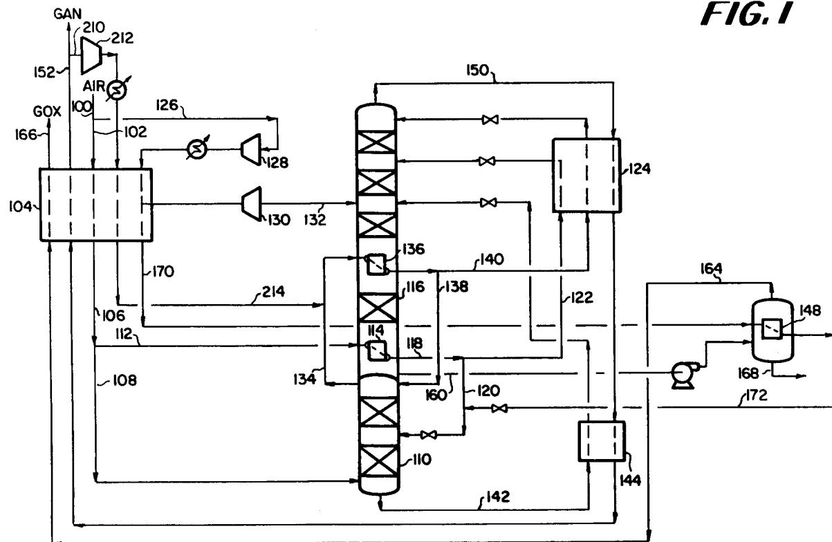
The present invention relates to processes for the cryogenic distillation of air at elevated pressures having multiple reboiler/condensers in the lower pressure column and has particular but not exclusive application to the integration of those processes with gas turbines.
