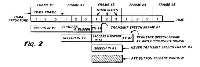
The present invention relates to trunked digitised voice transmission systems and more particularly to radio disconnect and channel access signalling in such systems. Particular application is found wherever digitised electrical signals of any type are to be transmitted in a constrained bandwidth having a limited number of signal transmission channels. The present application is particularly advantageous in trunked TDMA radio communications.
