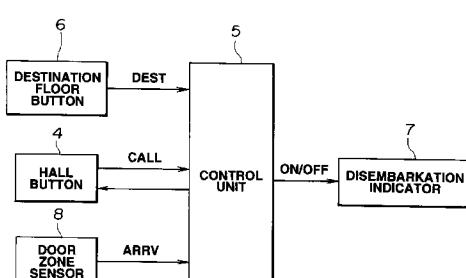
The present invention relates generally to an indicator system and method for an elevator.
