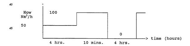
Basic flow is 50 Nm $^3$ /h at 2% O $_2$  content. Surges of 100 Nm $^3$ /h consumption at 2% O $_2$  occur during 10 mins every 4 hrs.
