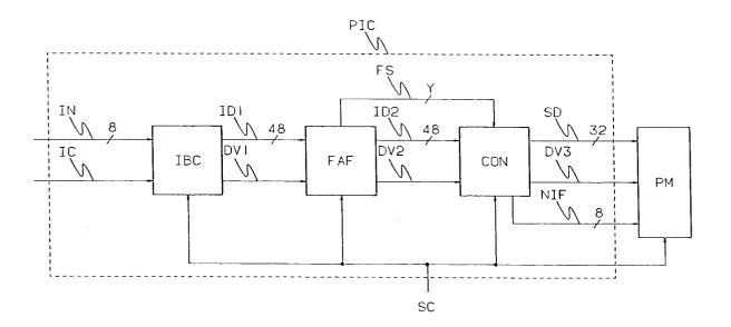
The present invention relates to an interface circuit for deriving from an input datastream synchronous with an input clock signal a system datastream synchronous with a system clock signal, the difference between the frequencies of said input and system clock signals having an unknown value comprised between predetermined bounds, and said interface circuit inserting stuffed data in said system datastream at a stuffed datarate dependent upon said difference.
