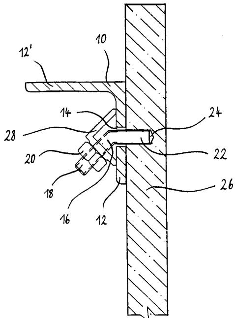
The present invention relates to a system for attaching panels onto a wall of a building and in particular to a system for attaching stone panels such as granite panels onto the walls of high rise buildings.
