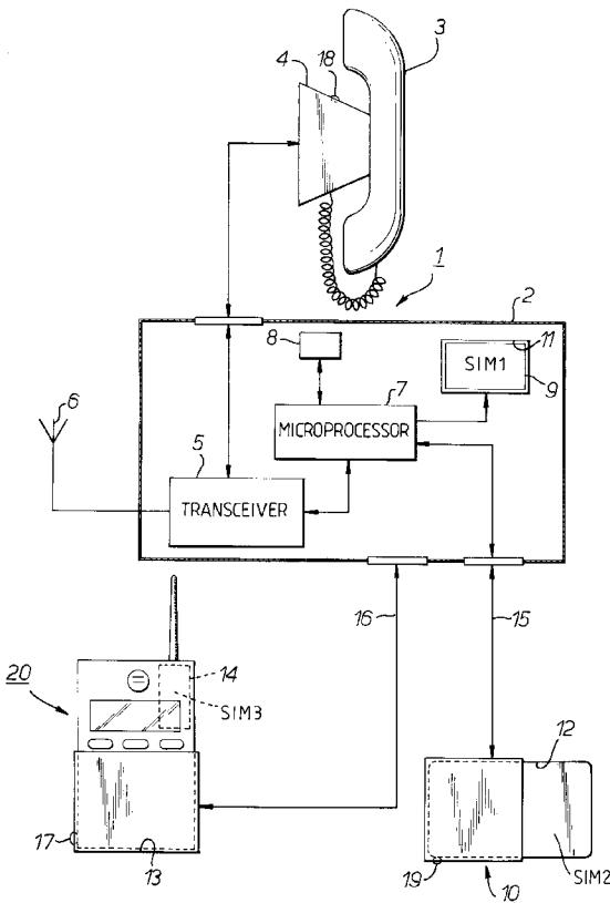
This invention relates to a radio arrangement and, more particularly, to a radio arrangement including means for removably receiving a memory module for storing information.
