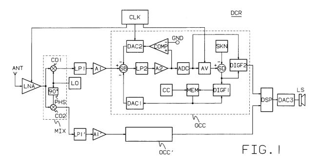
The present invention relates to an offset correction circuit for removing offset from an input signal being input thereto in assigned time slots.
