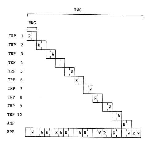
Transmitting ports: 1, 2, 6, 8, AMP, BPP Receiving ports: 3, 5, 7, 9, 10, BPP Idle ports: 4
