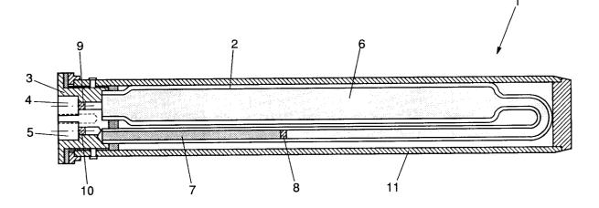
This invention relates to a filter for cleaning gases, comprising a quick-change coupling with an inlet and an outlet channel, and a hollow filter material housing filled with filter material through which, in operation, the gas to be cleaned flows.
