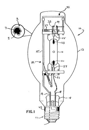
This invention relates to high intensity discharge lamp. More particularly this invention relates to such lamps having a coating of phosphor on the interior surface of an outer envelope.
