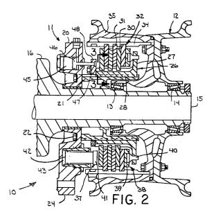
The invention herein described relates generally to a wheel and brake assembly and especially to one that is useful in landing gear for aircraft.
