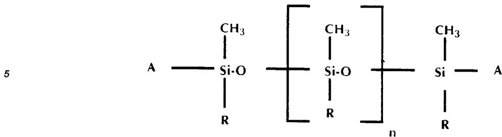
wherein R is an alkyl, alkenyl or aryl, or an aryl group substituted with an amino, hydroxy, mercapto or alkyl or alkenyl group, the functional group A is an alkene or alkyne, an alkene or alkyne substituted with an alkyl or aryl, and n is a number of from about 2 to about 350.
