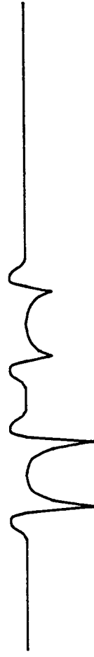
Fig. 7E EMITTER VOLTAGE OF TRANSISTORS 34 (IMAGE QUALITY CORRECTION SIGNAL)
