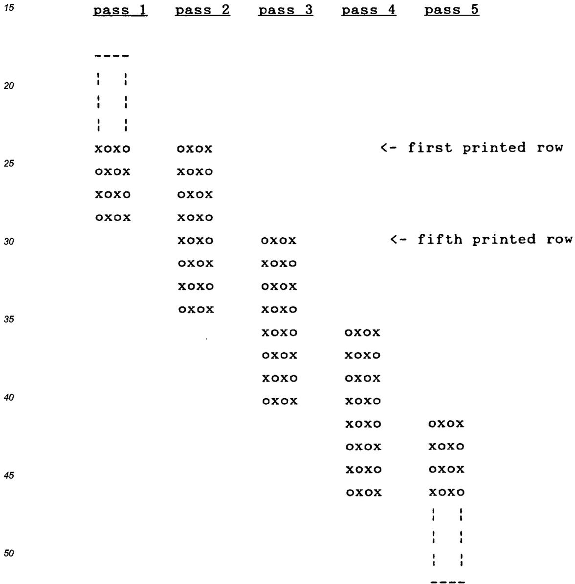
In this mode, the pen uses the same pattern all down the page, but the mask is different in different portions of the pen: "pattern 1" for nozzles one through fifty (represented in the abbreviated drawing by the lower four positions in each eight-nozzle group); vs "pattern 2" for nozzles number fifty-one through one hundred (represented by the upper four positions in each group).
