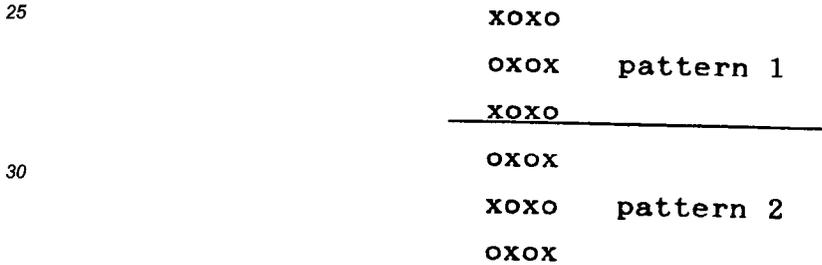
For an autorotating case, either "pattern 1" or "pattern 2" may be used all down the pen. Thus the paper advance turns one simple pattern into a space-rotated mask "automatically". In the shorthand notation introduced above, the pen provides the following periodic behavior as the paper advances.
