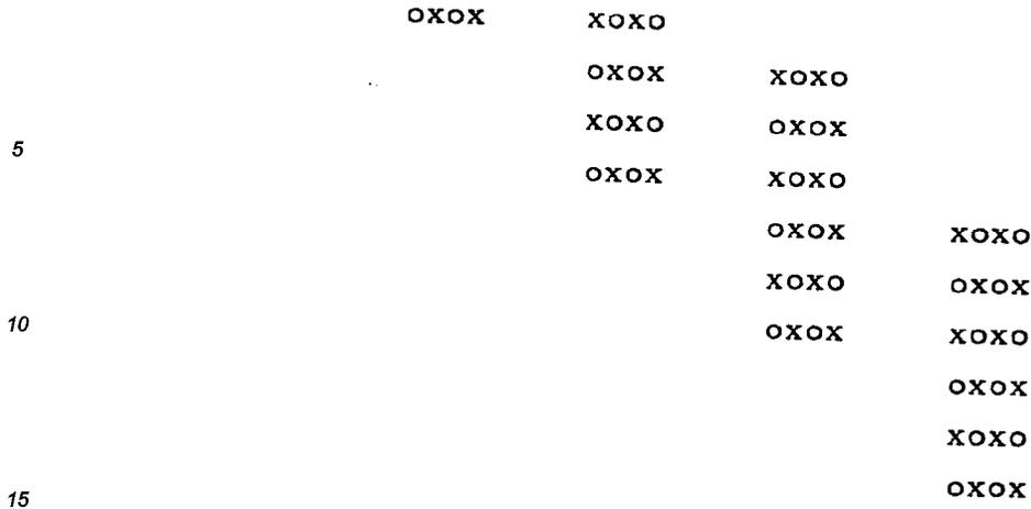
(This diagrammatic example symbolizes a real case of, for instance, three passes, a total of ninety-six nozzles used in the pen, thirty-two nozzles used in each of three sections of the pen, thirty-two-nozzle printing-medium advance -- and a basic-pattern cell three pixels tall. In algebraic notation,  $\frac{m_p}{h_c} = 32/3$ , a nonintegral ratio. This three-pass mode is discussed in the next section.)
