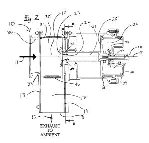
This invention relates to a variable area convergent-divergent nozzle and particularly to a variable area convergent-divergent nozzle acting as part of an attitude control system for a vertical take off or landing aircraft.
