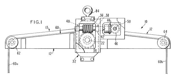
This invention relates to improvements in the lifting of loads of various kinds and, more particularly, to apparatus which allows for orienting a load after the load has been lifted above the ground.
