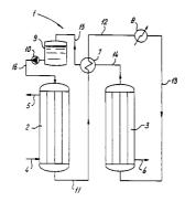
The present invention relates to a process for the separation of an unsaturated hydrocarbon from a fluid mixture with other hydrocarbons wherein in a first stage the unsaturated hydrocarbon migrates through a membrane to a carrier fluid and in a second stage the unsaturated hydrocarbon is separated from the carrier fluid and removed.
