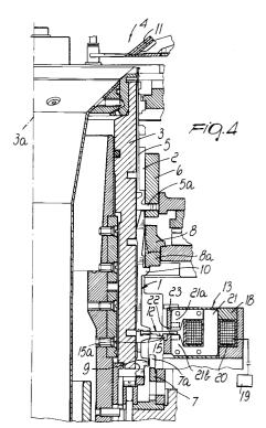
The present invention relates to a needle selection device for circular knitting machines for manufacturing socks, stockings or the like.
