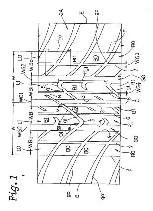
The present invention relates to a pneumatic tyre capable of reducing pass-by noise while maintaining steering stability, wet grip performance and other running performances.
