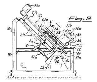
The object of this invention is an automatic machine for the production of rounded and/or substantially rectilinear bevels at the corners of flat sheets made of various materials.
