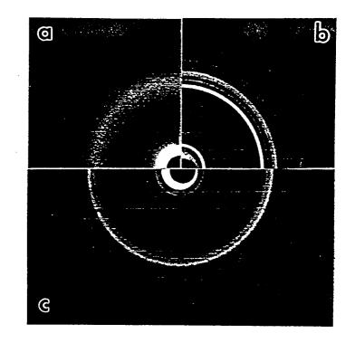
Wide-angle X-ray diffraction patterns: a) PANI/DBSA; b) SG; c) PANI/DBSA/SG
