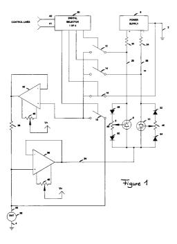
The invention relates to a current source and sink, and more particularly to a precision tracking, switchable bipolar current source/sink with ground clamping (zeroing) at the discrete circuit level.
