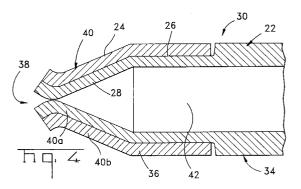
The subject invention relates to an improved electrical terminal and a method of making the same, and in particular terminals having increased contact force added by an additional back-up spring.
