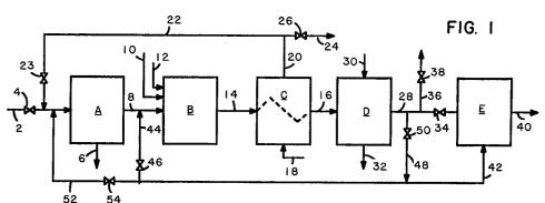
The present invention is directed to a process for producing partial oxidation products by the reaction of ethylene or propylene and an oxygen-containing gas in the presence of a suitable catalyst, and more particularly to a vapour phase process in which a hydrocarbon partial oxidation product is produced by contacting an ethylene stream or a propylene stream containing propane as an impurity with an oxygen-containing gas in the presence of an appropriate oxidation catalyst.
