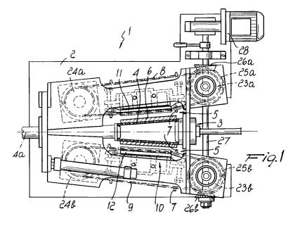
The present invention relates to a machine for cleaning cops or supports of spools of thread for the textile industry, particularly for cleaning frustum-shaped cops, cops or supports for "Soleil" spools, and "Ring" cops.
