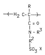
wherein R is H or  $CH_3$ , X is H or metal cation,  $R^2$  is  $C_{1-8}$  alkyl or phenyl and  $R^3$  is H or  $C_{1-4}$  alkyl.
