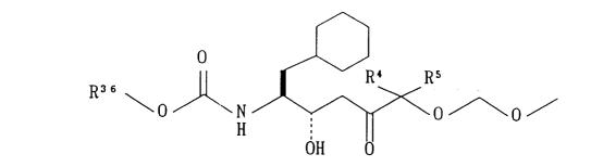
wherein  $R^4$ ,  $R^5$  and  $R^{36}$  are as defined above, and reducing the obtained compound using a boron hydride compound in the presence of a lower alkylcarboxylic acid to stereoselectively produce a compound of the formula
