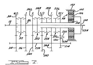
This invention pertains to the arrangement of gears, shafts, and synchronisers of an automotive transmission, especially to such a transmission of the type having a countershaft or layshaft disposed parallel to a power input shaft.
