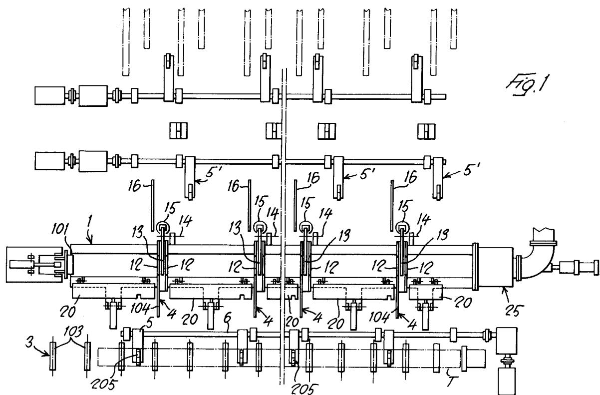
The invention relates to a method and a device for quenching, particularly for steel tubes or similar.
