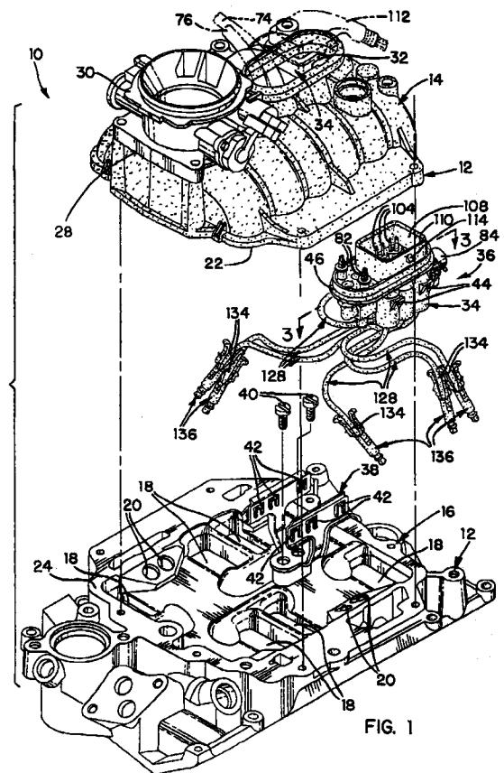
This invention relates to an integrated fuel and air induction system for an internal combustion engine.
